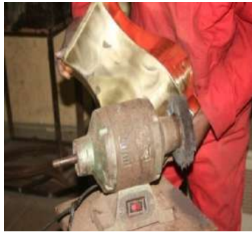
Figure 10: Polishing Lampshade-Stand in Metal Design Studio, University of Benin, Nigeria.
