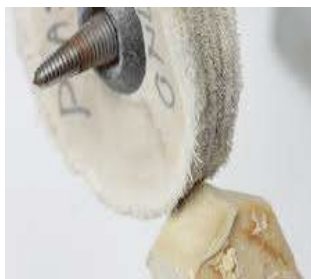
Figure 7: Impregnating the Polishing Wheel with Polishing Compounds.
