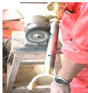
Figure 8: Polishing with Motor Secured on a Bench in Metal Design Studio.
