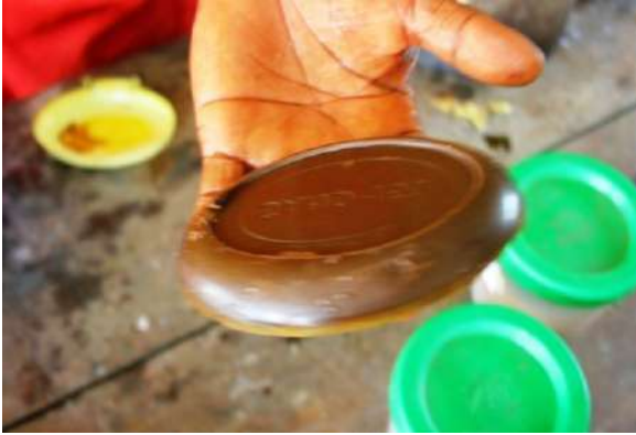
Figure 17: A Blended Bar Polishing Compound.
