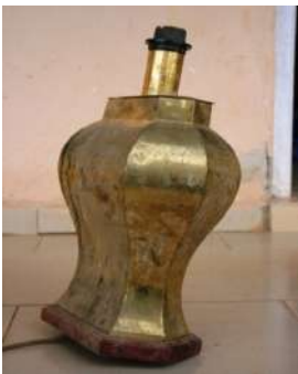
Figure 9: The Surface of a Brass Lampshade-Stand before Polishing Operations is Applied.
