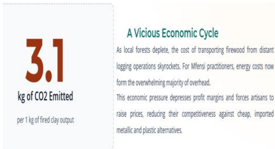
Fig. 12(b): Firing characteristics of systems in Regions of Ghana and estimated emitted CO 2
