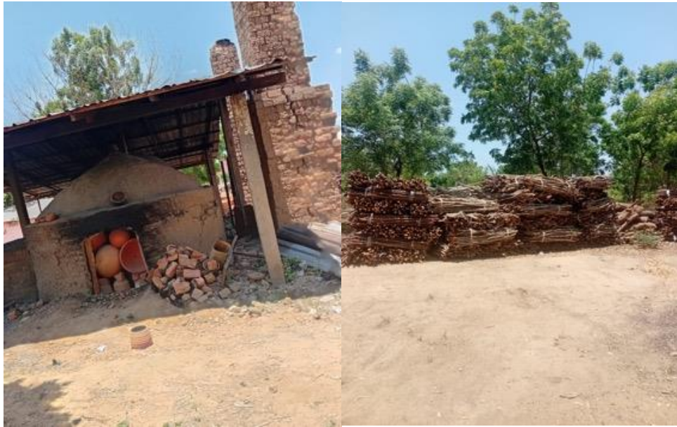
Fig. 13: Currently traditional firewood Kiln in practice and packed firewood in Ghana
